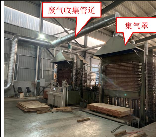
热压机集气罩+废气收集管道
